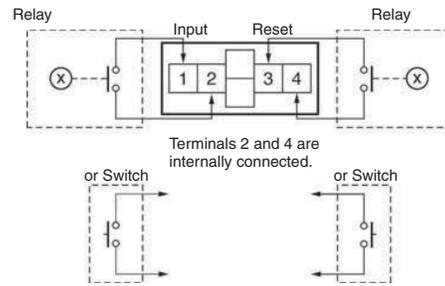
**Note:** Use Relays and Switches that have high contact reliability because the current flowing from terminals 1 or 3 is small. It is recommended that OMRON's G3TA-1A/ID be used as the SSR.
